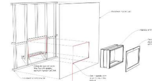
**IMPORTANT** → Insulation must be securely wrapped around the firebox body before placing inside opening
