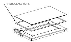
Refit the glass retainers by repeating step 1 to 2 in reverse. 7. FITTING A NEW DOOR SEAL
