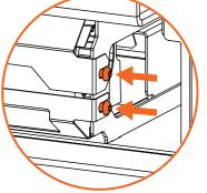
5. Lift up and pull the fan shielding assembly out.
