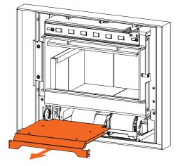
6. The fan housing can then be removed.
