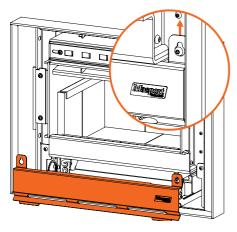
Remove the receiver mount screw with a 5mm hex key. The receiver box can now be carefully pulled out from the heater.
