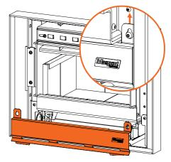
3. Disconnect the power lead to the receiver box.
