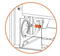
Disconnect cables and replace receiver unit. To install new receiver unit, connect cables and repeat steps 1-4 in reverse order.
