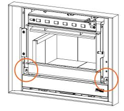
Access panel can then slide upwards and be removed from heater.
