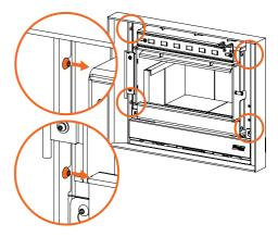
With main fascia removed from the heater, the extended fascia can hook onto its inside edge. With the extended fascia in place, reinstall the main fascia onto heater, press both the main and extended fascia into the front face of the enclosure before re-tightening screws with a 5mm hex key.
