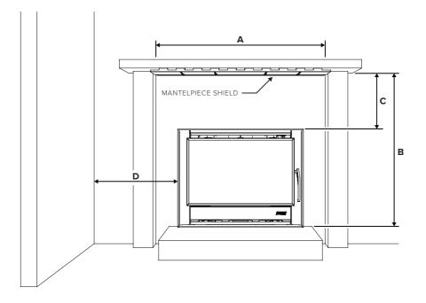
Refer to this section for clearance requirements and instructions if heater is to be in a masonry installation. For variations to clearances relative to a combustible mantelpiece refer to AS/NZS 2918 Clause 3.4.2.
