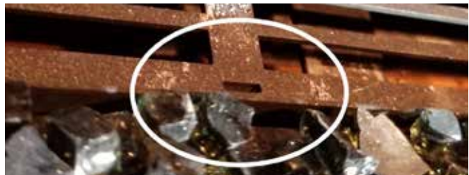
Burner covered with Fireglass and glowing wool
