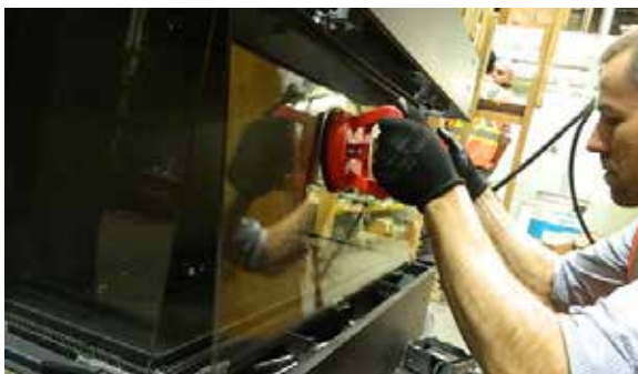
Handle front panel with supplied vacuum clamps
